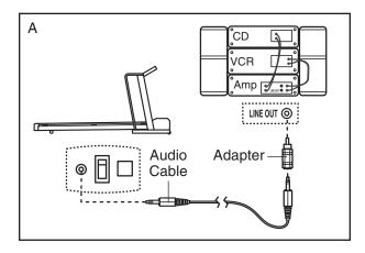
B. Plug one end of the audio cable into the jack on the front of the Incline Trainer near the power cord. Plug the other end of the cable into the included adapter. Plug the adapter into an RCA Y-adapter (available at electronics stores). Next, remove the wire that is currently plugged into the LINE OUT jack on your stereo and plug the wire into the unused side of the RCA Y-adapter. Plug the RCA Y-adapter into the LINE OUT jack on your stereo.
